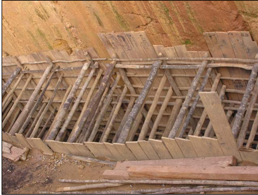
Figure 15.1c. Photo illustrating the support used by the artisanal miners to hold the walls of the main shaft from collapsing.
