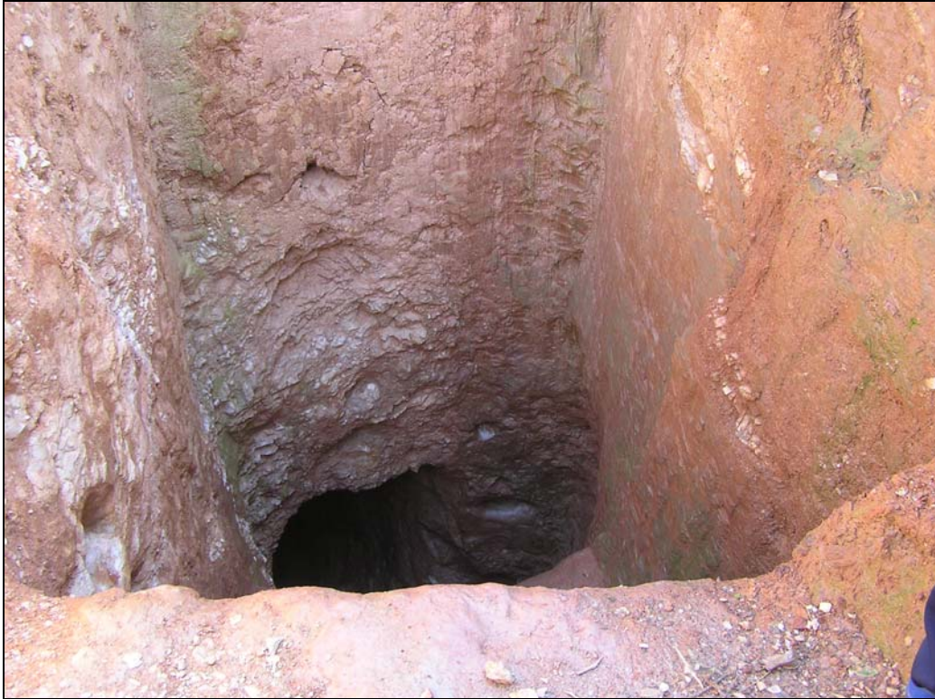
Figure 9.0i. Photo of a pit and tunnel on the Golgotha artisanal gold mine; note the quartz veins in the pit walls.
