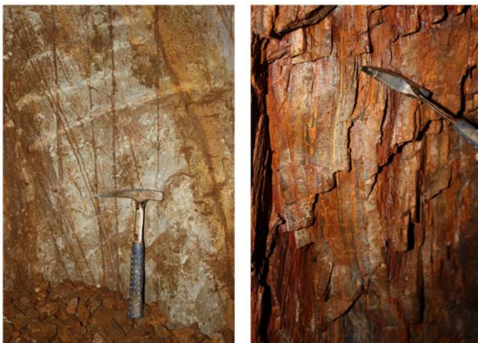
Figure 6: Photographs of meta-volcanosedimentary hangingwall (left, facing approximately southeast) and BIF (right, facing upwards, with the top of the photograph in the southeast) in an old Belgian era adit. The BIF is highly sheared parallel to the lithology contacts.
