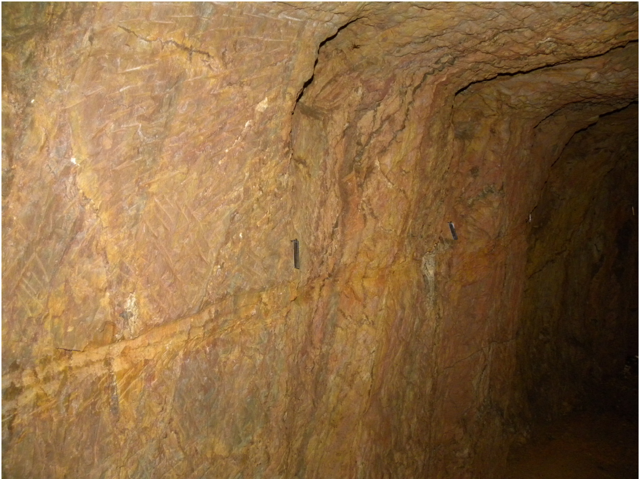
Figure 3) KGL Somituri Project – Location of continuous horizontal channel samples on adit wall.
