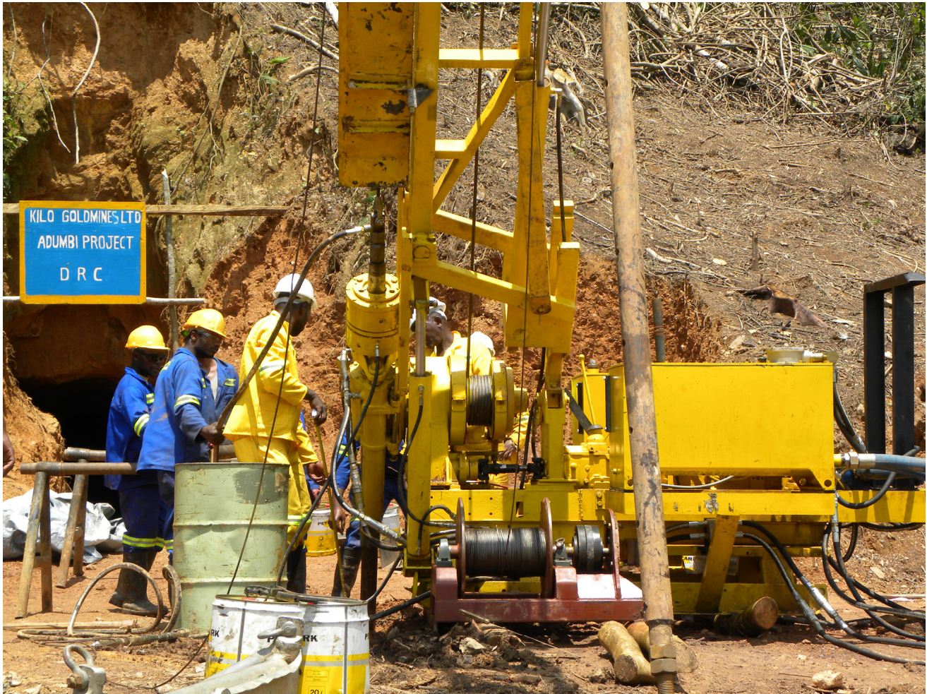
Figure 1) KGL Somituri Project – Diamond drilling at the Adumbi site.
